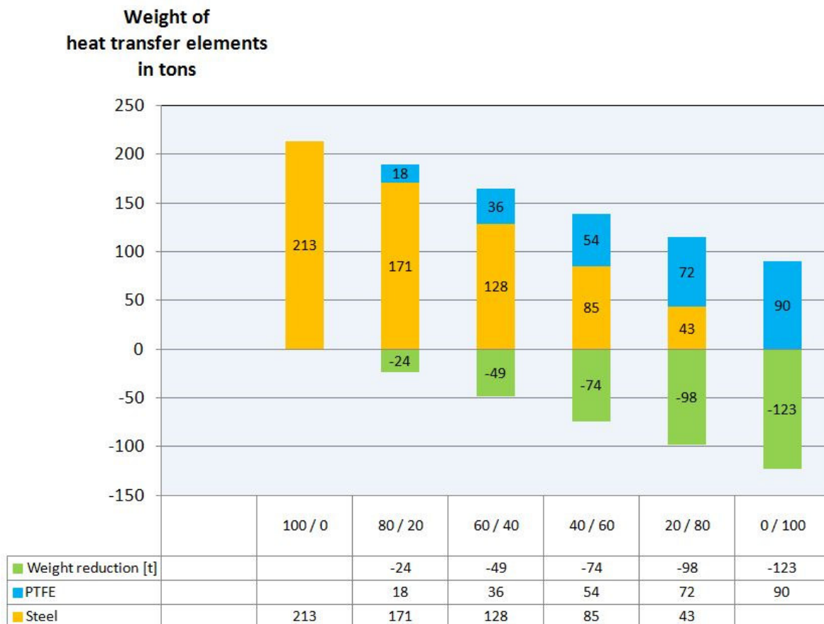
Fig.9: The potential for weight reduction of Ljungstroem® rotors by replacing steel packages with PTFE combs -keeping the same level of heat transfer capacity- is significant: Just as an example, if a rotor with twenty meters in diameter and with a height of the heat transfer elements of one meter, a complete replacement of the steel packages by PTFE combs will reduce the rotor weight by about 125 tons (!): From left to right in Fig.9: successive replacement of steel packages by PTFE combs.
