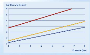
Test Conditions: Piston rings made of PTFE, dimensions:  $\emptyset$  48 x  $\emptyset$  60 x 6 Piston rings not run in Static test T = 100 °C Medium: Air
