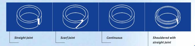
Guide rings with scarf joints provide the advantage of fully running across the cylinder contact surface, thus causing no "markings" on the surface unlike the straight joint.
