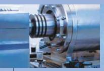
Test rig for rotary shaft seals with PTFE sealing lip for testing various parameters.
