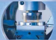
Test rig for long-term wear rates of PTFE compounds with various sliding mates.
