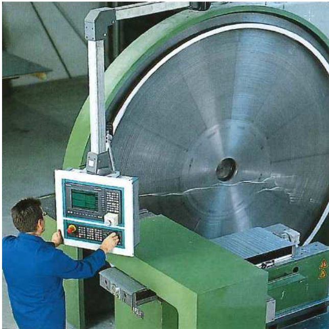
Figure 50: the finished test piece is processed on a lathe
