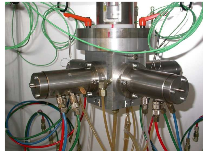
Figure 28: test bench for seals in direct-injection gasoline systems
