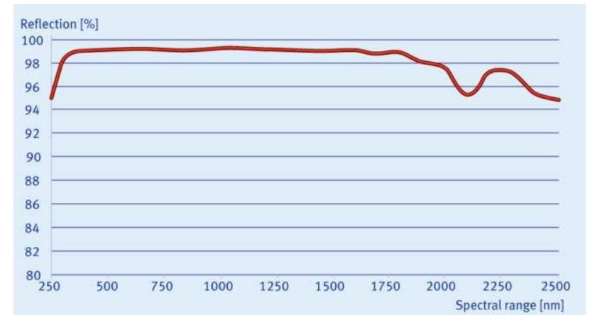
Figure 20: the reflection spectrum of porous PTFE
